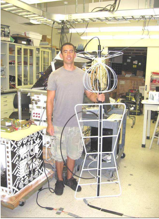
FIG. 11: Christian Miki holds an example of a fully tested production model of current configuration of hybrid testbed vertices, combining both batwing and discone antennas that fit together into the 2m deep by 24” diameter auger-bored borehole. 6 sets of these antenna pairs have been already constructed and tested.
