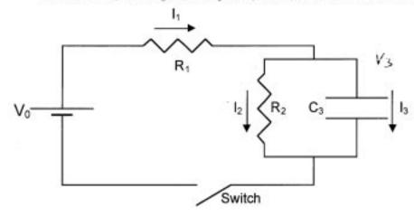
(a) What are the three currents  $I_1$ ,  $I_2$ , and  $I_3$  at t=0, right after the switch is closed?  $V_3 = C \implies \mathcal{T}_2 = C$
