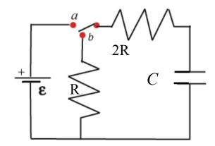
6. (5pts) Just after the switch (a) is closed, what is the current drawn from the battery?
