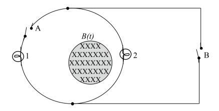
Two light bulbs are connected to opposite sides of a circular loop of wire as shown. A changing magnetic field is confined to the smaller gray area. All switches are initially open. When switch A is closed both bulbs are lighted.
